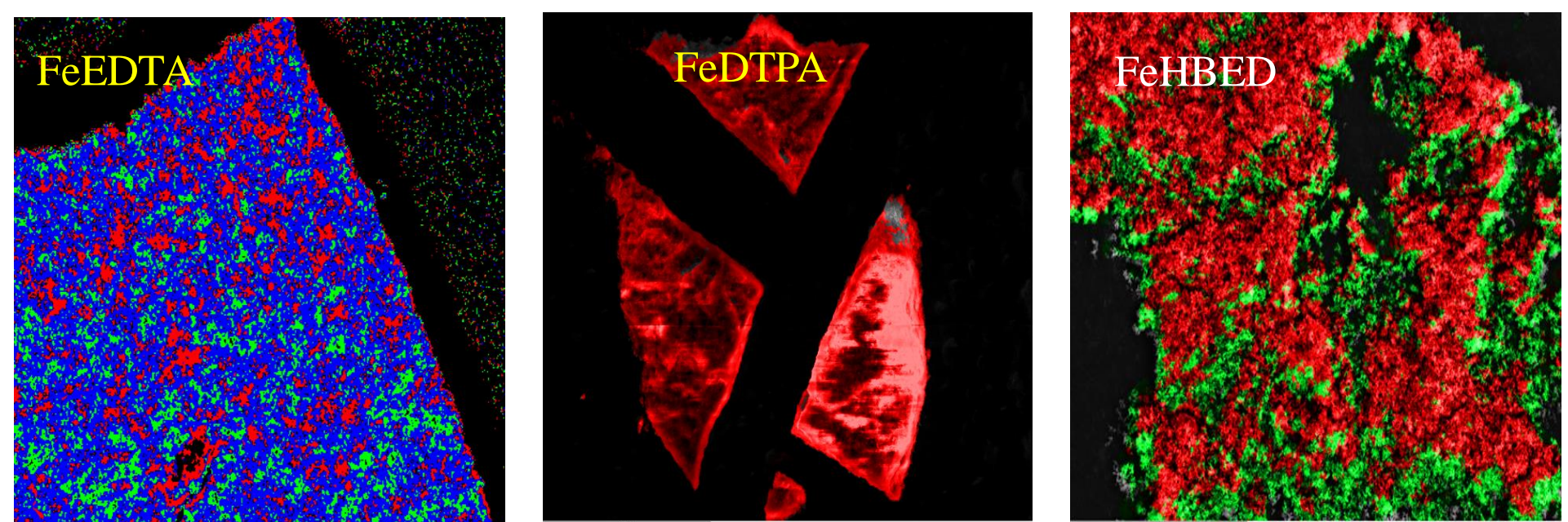
Fig. 5. SEM-EDX composition images of the precipitates collected on the surface of filter papers of 5 mM NaHCO 3 containing nutrient solution with different Fe sources. Various colors represents presence of elements at different depths in the sample.
