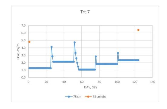
Irrig 240 mm, EC<sub>irri</sub> – 8 dS/m Drainage – 67 mm
