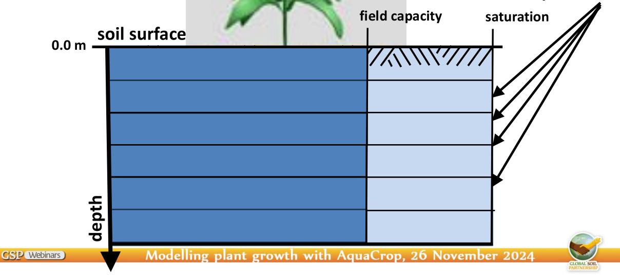
to simulate the convection and diffusion of salts, a soil compartment is divided into a number of cells in which salts can be stored compartments cells field capacity saturation 0.0 m a cell is essentially a representation of a volume of pores with a certain diameter diameter of soil pore micro pores maçro pores Modelling plant growth with AquaCrop, 26 November 2024 Webinars
