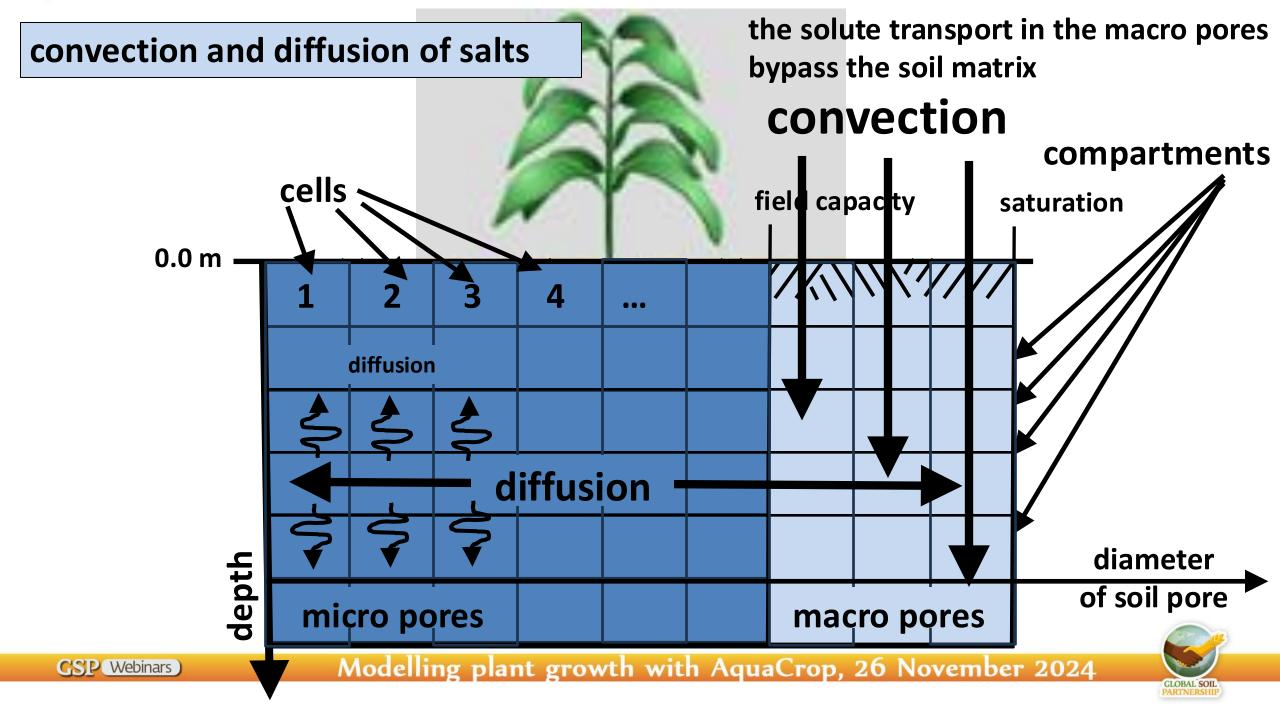
the driving force for the diffusion process is the salt concentration gradient that exists between the water solution in the adjacent pores
