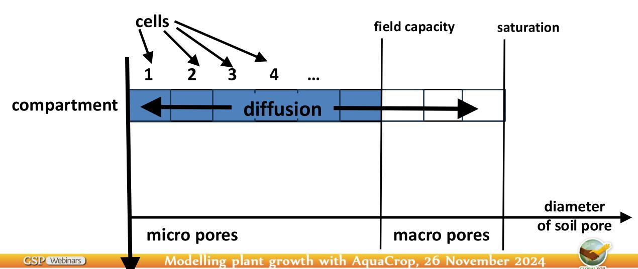
the driving force for the diffusion process is the salt concentration gradient that exists between the water solution in the adjacent pores
