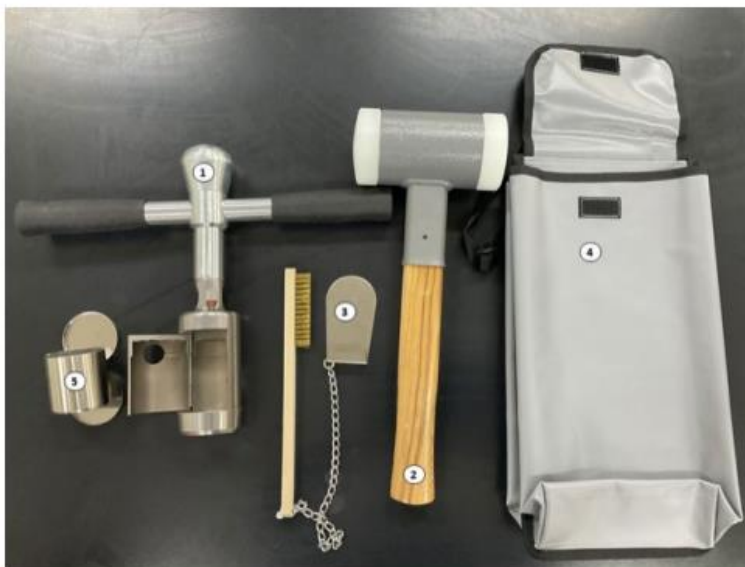
Figure 2. Field sampling set (this represents one possible device setup and others are possible, such as those with only a ring and a hammer)
