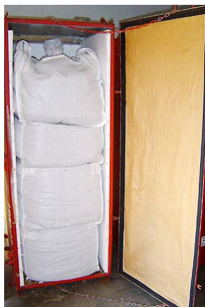
Figure 1. Filling level full (600kg approx.) headspace 230mm
