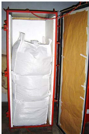
Figure 2. Filling level \frac{3}{4} (450kg approx.) headspace 430mm
