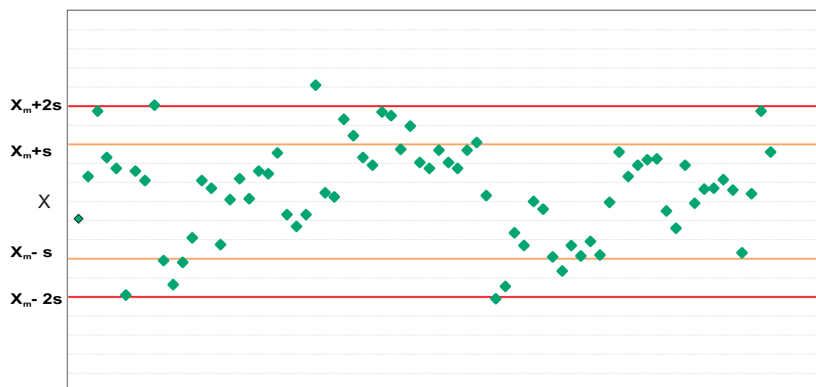
Figure 25: Example of Control chart of in-house material [naturally contaminated coffee sample, (4.99 + 0.58 µg/kg, n=20), n=78], SOP 039 ed. 03, rev. 02 (Immunoaffinity column clean-up and HPLC)
