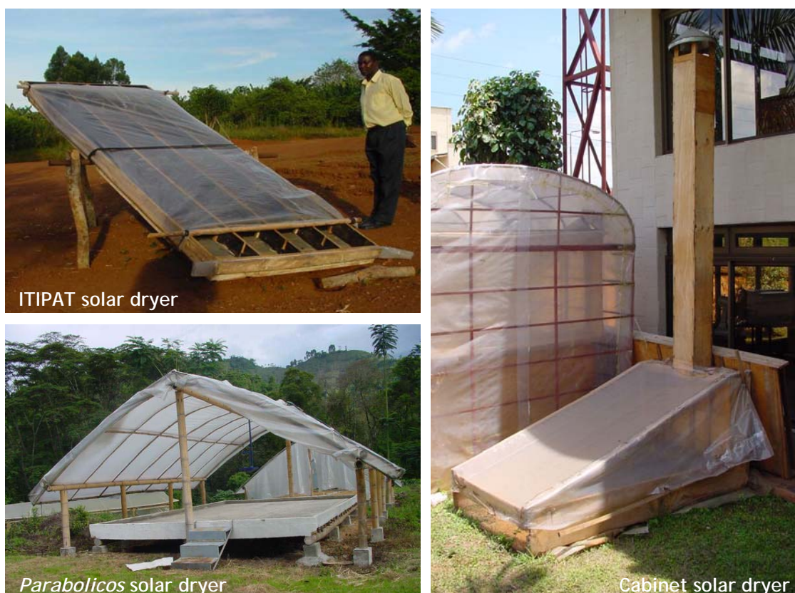
Image 4.2: Three solar dryer designs field-tested during the course of the project.
