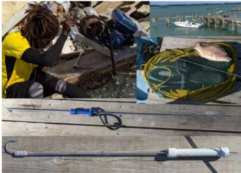
Figure 20. Fisherman fixing his compressor for use on his dinghy (top right) with long hose (yellow in net). He fishes with a spear or collect lobsters and conch with a hookah (authors).
