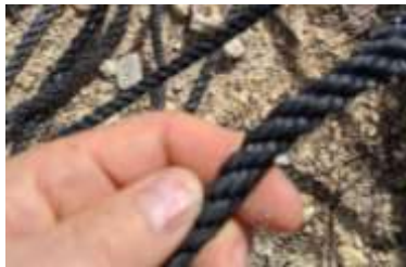
Figure 19. Common rope in use for pot fishery in Bahama, Three stranded polyethylene in black (authors).
