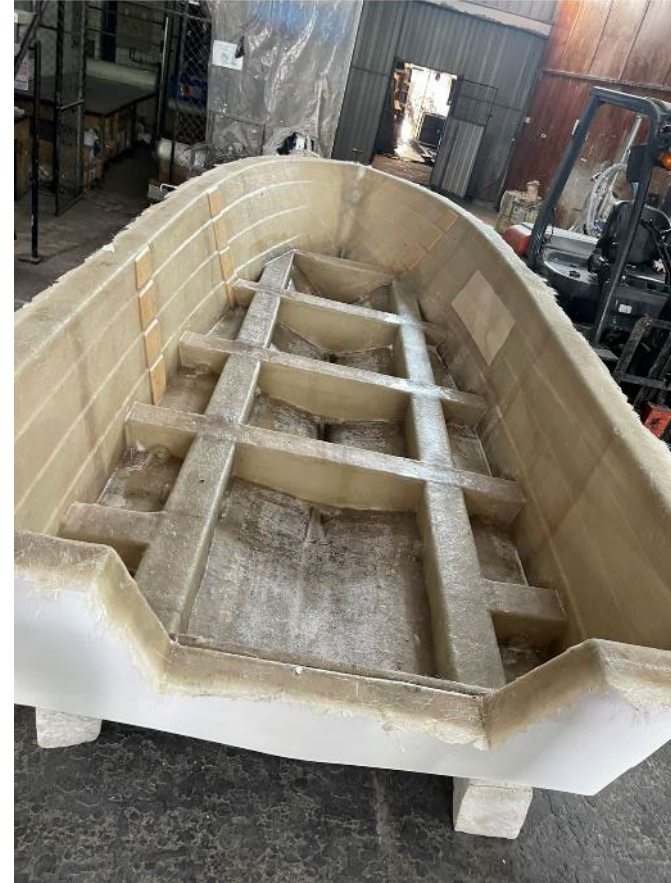
Proposed example of longitudinal girders giving the boat improved strength along the length
