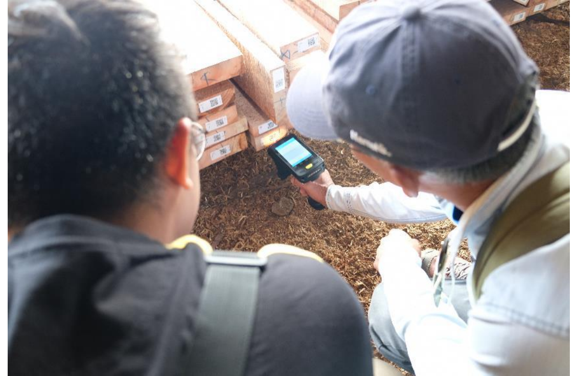
A handheld reader is used to scan QR codes attached to lumber produced from inventoried trees as part of a tracking system developed for timber traceability in the Philippines under an ITTO project. Photo: Forest Management Bureau
