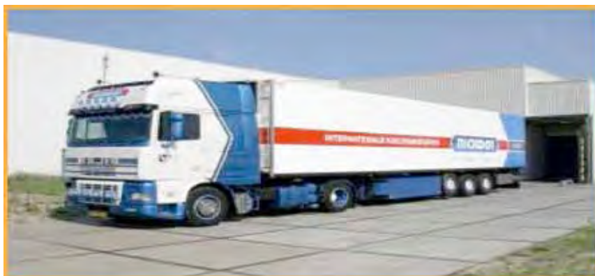
Figure 9: Long-distance meat truck (20 to 22 tonnes net load)
