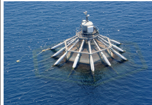
FarmOcean cage – semi-submersible, reduced surface exposure
