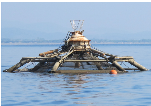
Sadco Shelf cage – rigid frame, submersible
