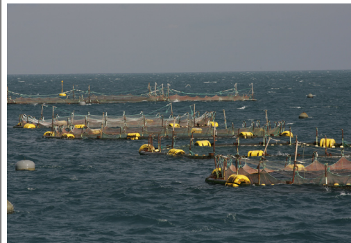
Bridgestone cage – flexible surface collar
