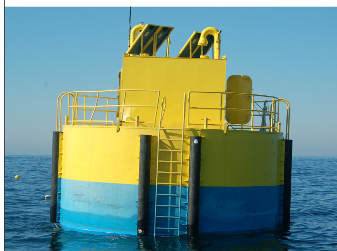
FIGURE 11 A 20-tonne prototype ocean farm feeder
