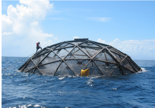
Aquapod – geodesic sphere, submersible
