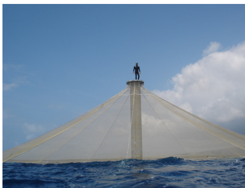
b) Sea Station SS3000 raised to rim-level on the Kona Blue farm site.
