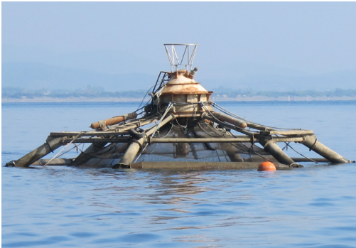
Sadco Shelf cage – rigid frame, submersible
