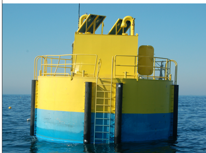
FIGURE 11 A 20-tonne prototype ocean farm feeder
