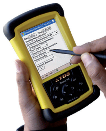
FIGURE 3.9 A typical waterproofed and ruggedized handheld data logger
