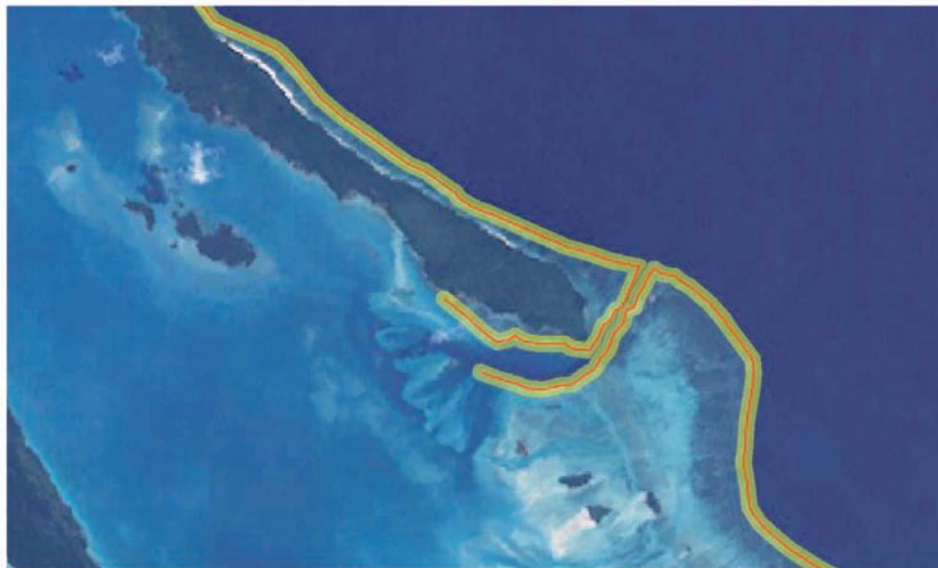
FIGURE 10.18 Example of identification and manual vectorization of reef edges and automatic buffering on the reef edges in the Maratua Atoll, Indonesia
