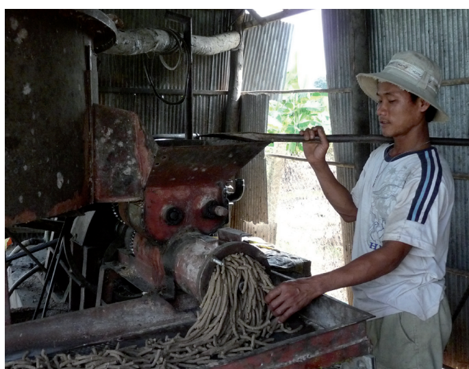
FIGURE 5 Extrusion of farm-made feed (FMF) for grow-out striped catfish ( Pangasianodon hypophthalmus )
