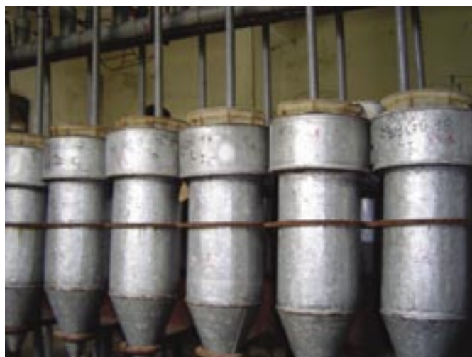
Small-sized incubation jars used in common carp and catfish hatcheries in Viet Nam
