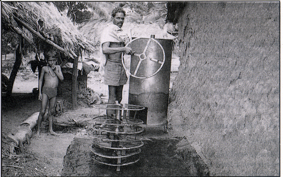
Fisherman operates improved smoking kiln.
