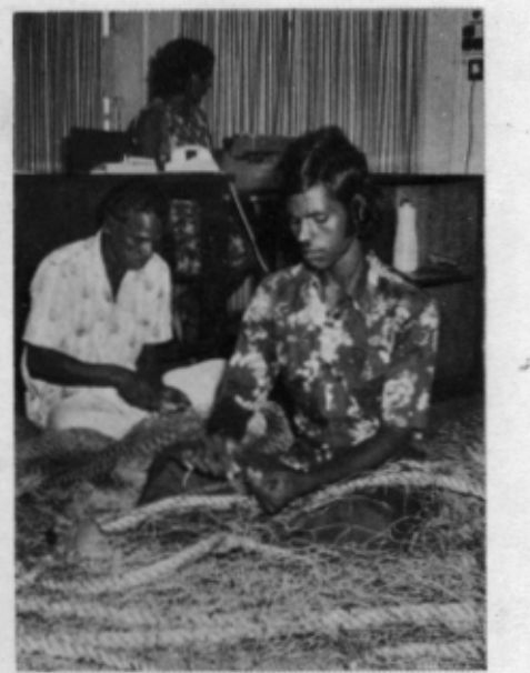
Two net-makers rigging a high-opening bottom trawl at the BOBP office in Madras for use in Bangladesh.
