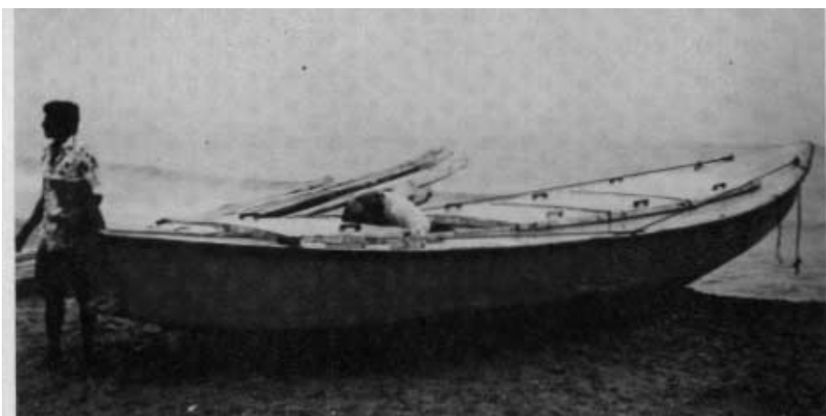
The two beachcraft prototypes selected for intensive fishing after the Ennore trials. IND 11 (below) is a kattumaram-type boat with buoyancy provided by polystyrene logs. IND 13 (above) is decked, and built of marine plywood.
