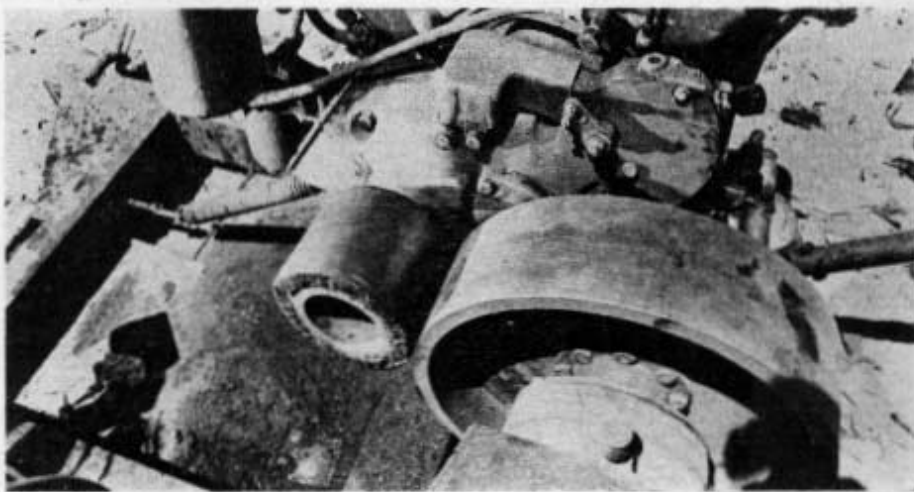
Above: The winch with its simple spooling arrangement and warp head. Below: The rubberized friction wheel is in contact with the driven wheel, combining the advantages of clutch and reduction ratio.
