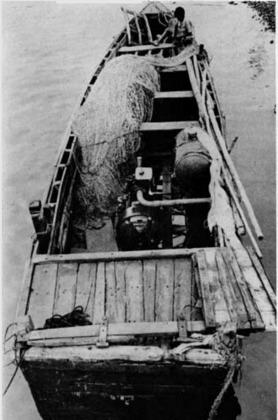
Motorized Nava with reversible gearbox and nets.
