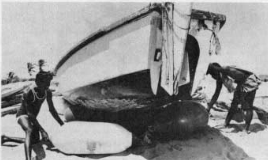
Inflatable fenders — one of the hauling devices for beachcraft described in BOBP/WP/5 7.
