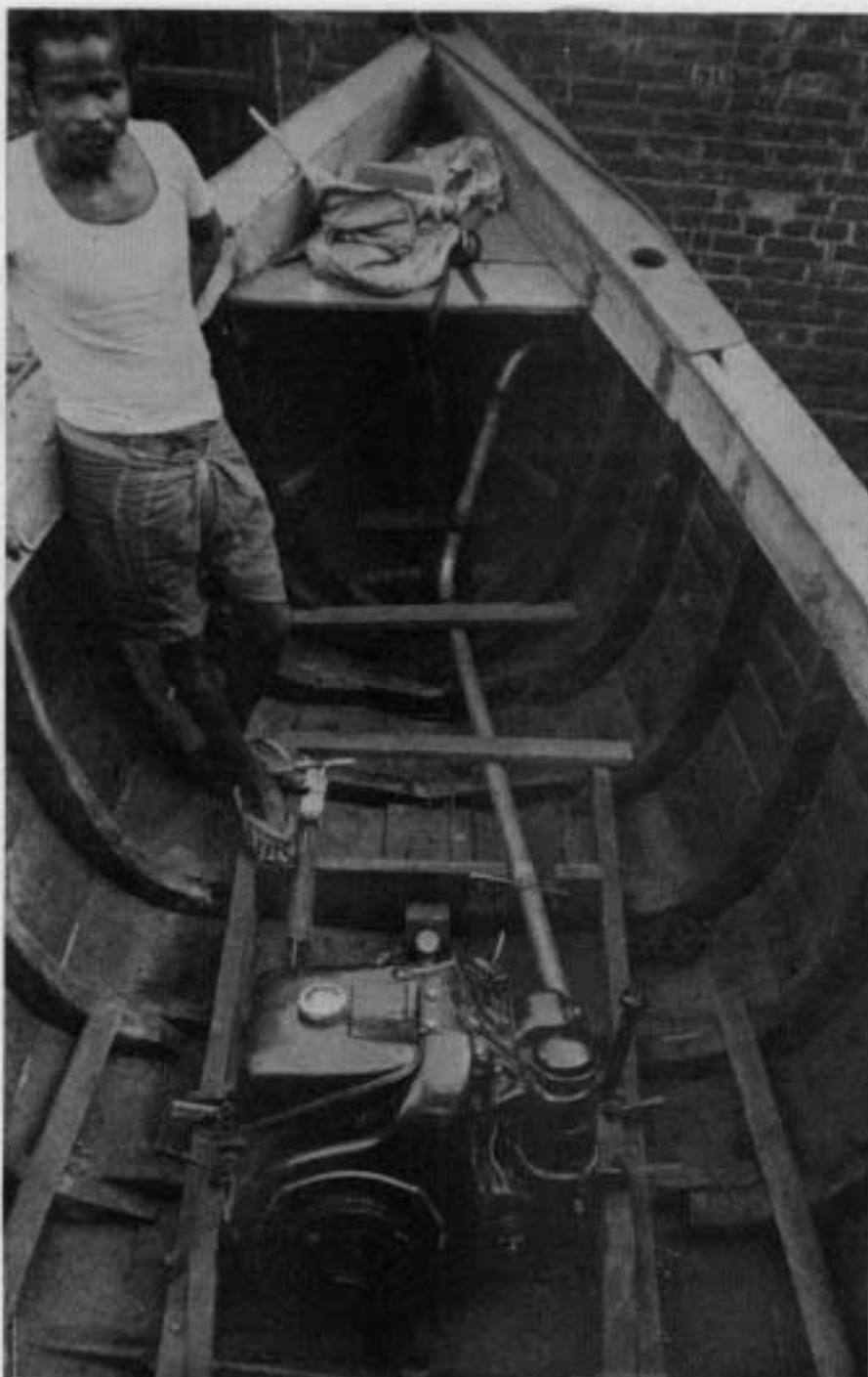
Inboard motorization of the dinghy in Kasafal, Orissa, tried out by BOBP.
