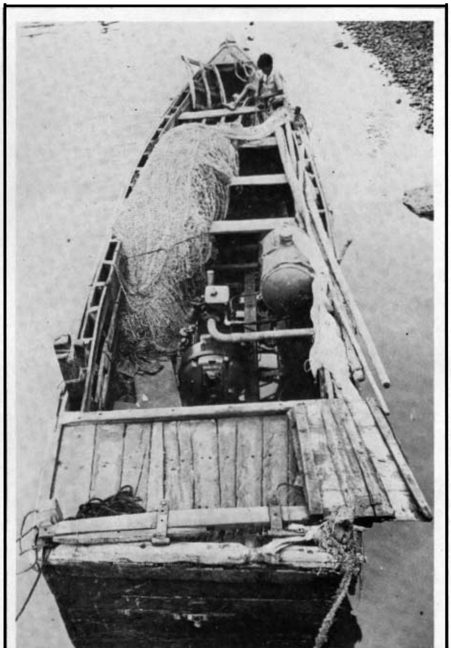
The motorized Nava of Kakinada. The motorization was carried out by the fisherfolk themselves on their own initiative.
