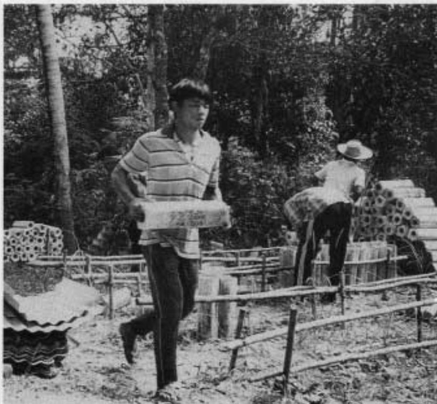
Manufacture of concrete pipes for oyster culture.
