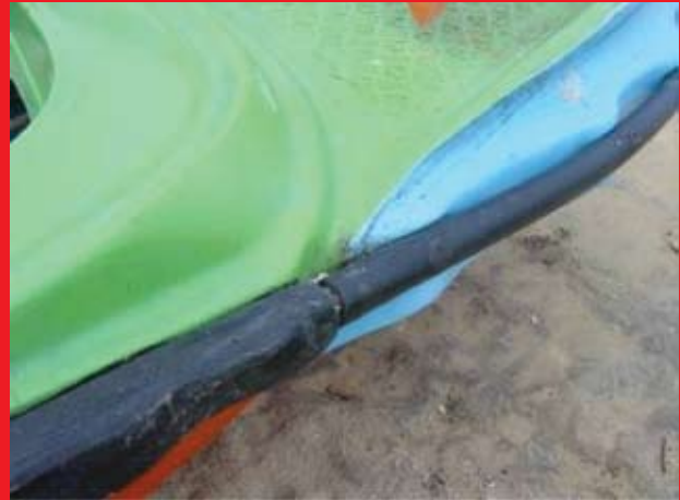
✔ Good overlapping the wood and the PVC-pipe of the fender on a 6-7m FRP boat. The wooden fender is 2" thick and the scarf is supported by the laminate of the boat.
