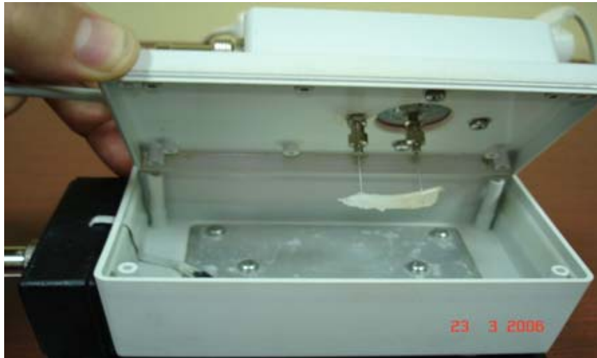
Plate 2. Fish muscle sample placed on needle electrodes of the measuring box.
