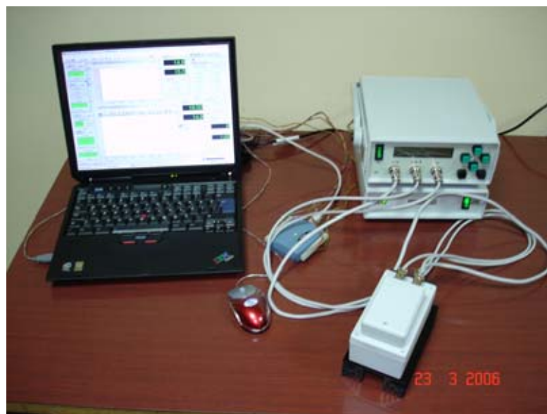
Plate 1. Instrument used for measuring muscle contraction speed.
