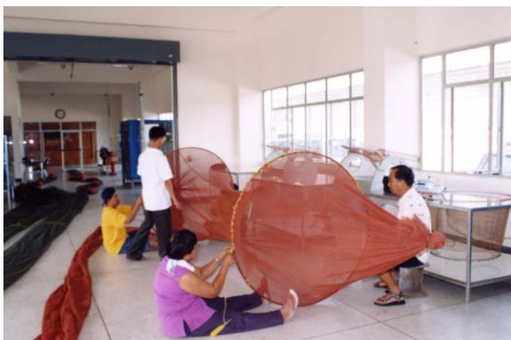
Figure 4. Participants constructing a JTED in the Fishing Workshop.
