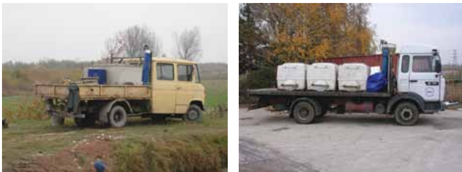
Lorries equipped for transporting fish within and between fish farms.
