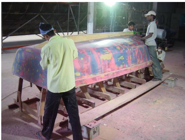
The plug almost finished. Bilge keels are ready to be added. Then the gelcoat will go on, and only the finishing and polishing will be left.
