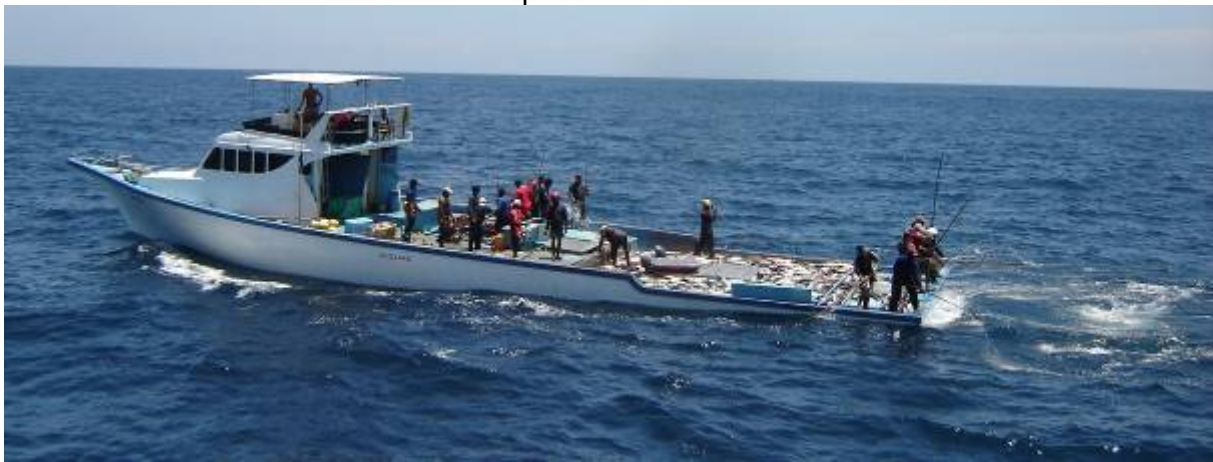
30 m Pole and line boat with a good catch of skipjack tuna. Note lack of freeboard aft.
