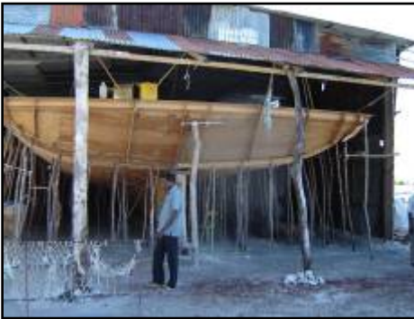
Mould transom of a 30 m pole-and line boat in Viligili village, Gaafu Alifu atoll
