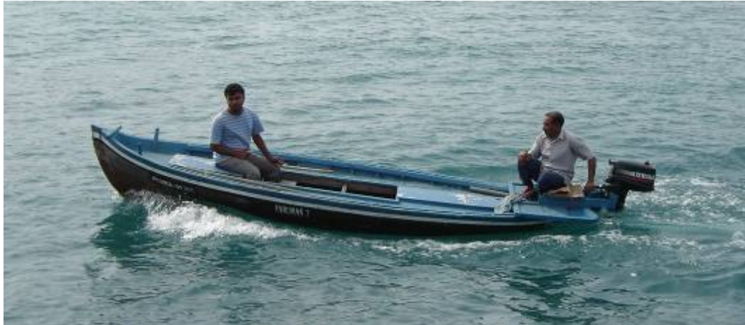
Bokura with 4 hp outboard engine. Note lack of freeboard aft
