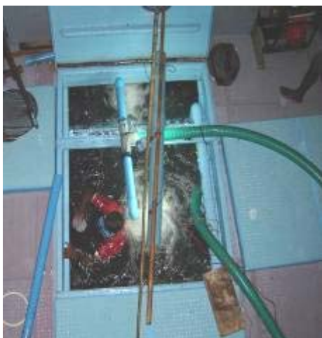
Baitwell hatch. The diver has unplugged one of the hull openings. Note plastic pipe to the left for insertion into the hole.
