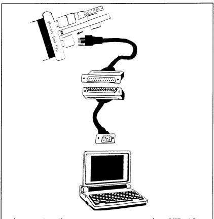
Figure 2. The way to connect the STD-12 plus to the portable computer.
