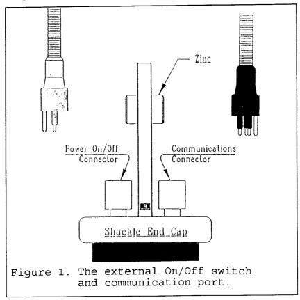
a- The communications port, is used to program the instrument as well as to recover the recorded data, it has a six hole connector (the black plug to insert has five golden pins and one silverish guide pin)
