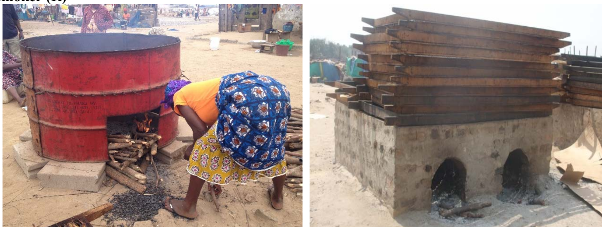
Figure 1. Traditional kilns for fish smoking in Ghana. Metal drum kiln (L) and Chorkor smoker (R)
