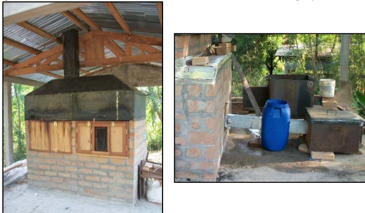
Figure 5. BIDUL/IRT kiln with indirect smoking system
