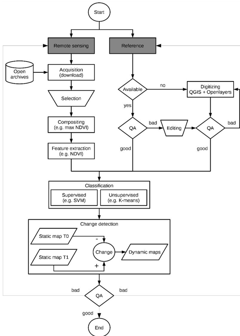
Figure 2. Schematic overview of the method applied to estimate land use and forest cover changes
