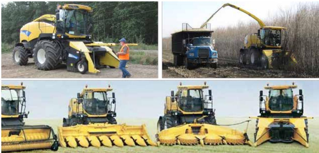
**Fig. 1:** Top left: A New Holland FR 9060 forage harvester with a 130 FB Coppice Header attached being prepared for a hybrid poplar harvest in Western Oregon. Top right: A FR-9080 forage harvester operating in a willow plantation at Auburn, NY in November 2012. Bottom: Examples of available headers for the New Holland FR 9000-series of forage harvesters including the 130 FB coppice header on the far right.
