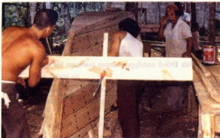
Local carpenters building an INS-S outrigger canoe in Gamo.
