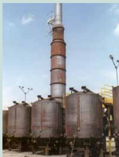
Metal kilns equipped with vapour incinerator for charcoal production in France
