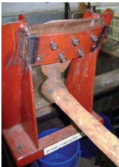
FIGURE 2 Clamping jig for hoes at the Kenyan Bureau of Standards
