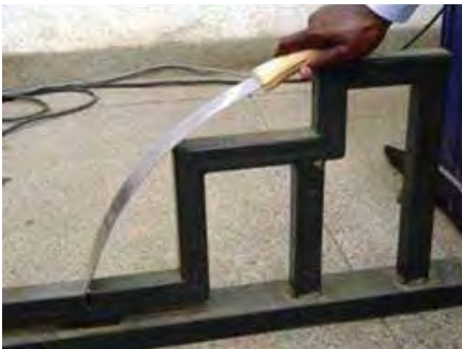
FIGURE 10 Apparatus for testing machetes at the Kenya Bureau of Standards
