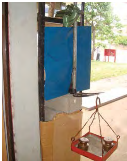
FIGURE 4 Clamping and loading arrangement for fork hoes
