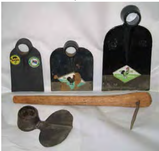
FIGURE 26 The original shape of the hoe (top right) and an even more worn example (bottom left)
