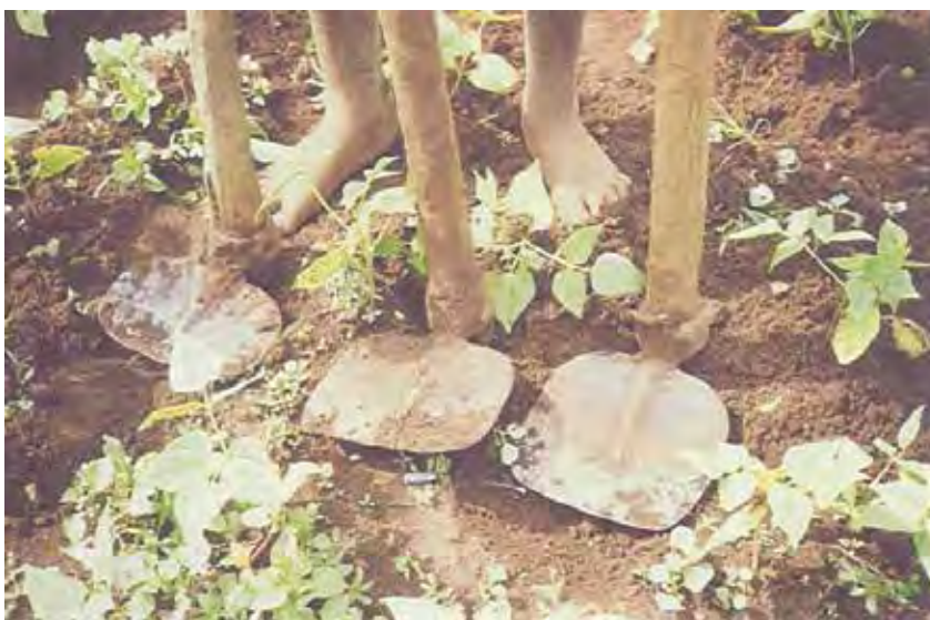
FIGURE 25 Used hoes in Burundi. The use of each is approximately (from left to right) “more than 5 years”, about 4 years and two years
