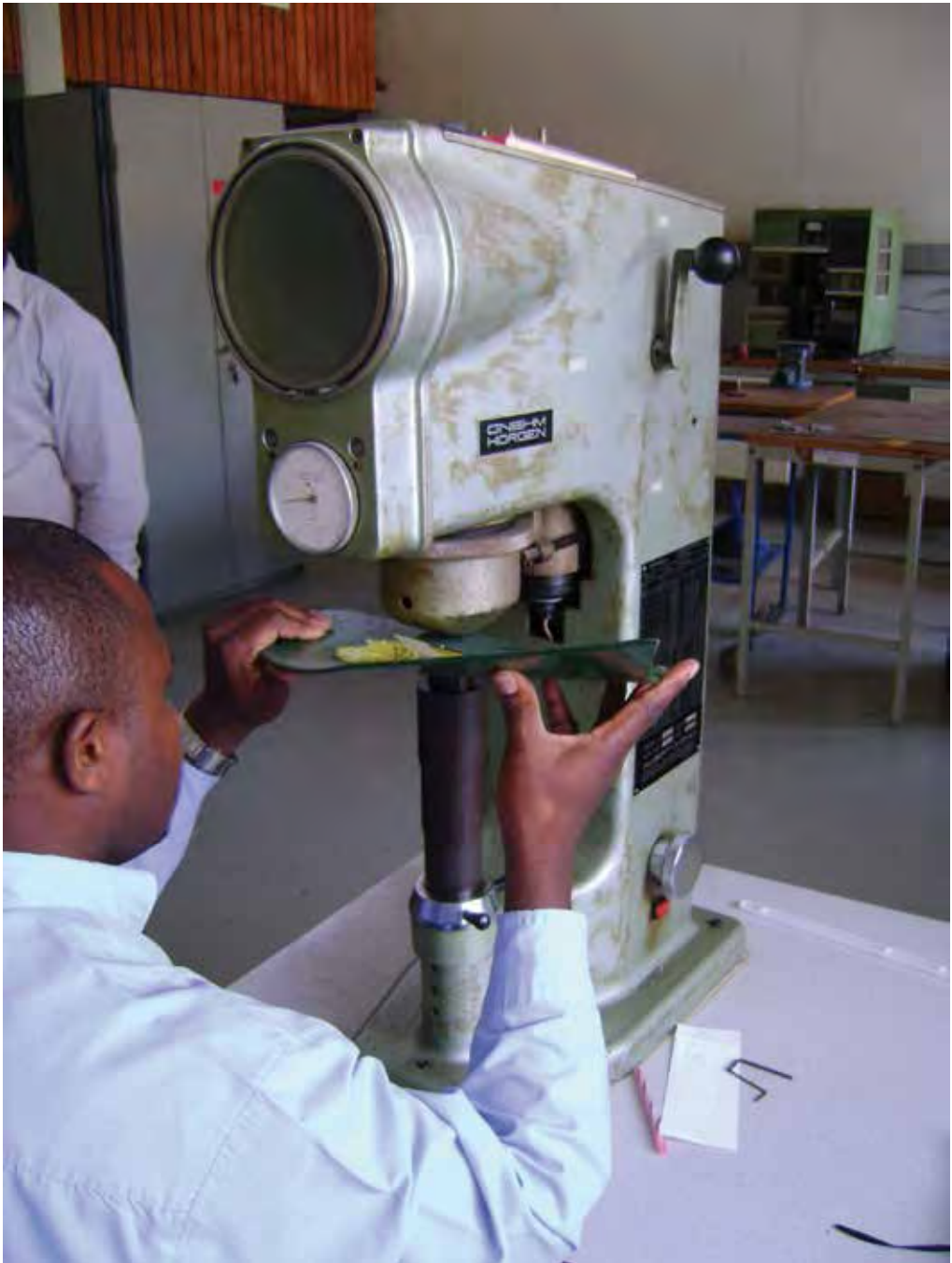
FIGURE 12 Hardness testing machine in the laboratories of the Kenya Bureau of Standards
