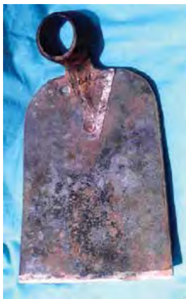
FIGURE 27 A “rehabilitated” hoe made by a blacksmith in Burundi. Although the blacksmiths are unable to make the “eyes” they can rivet on a strong new blade
