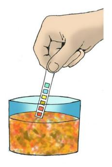
Then it can be pumped into storage tanks and stored for at least 6 months, or even more. Excessive use of acid should be avoided, primarily to keep production cost as low as possible. In the storage tanks pH should also be checked regularly (e.g. every week), and eventually corrected by adding more acid if needed.
