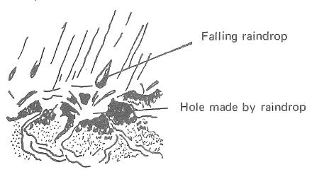
Around the house, the water that falls from the roof makes holes and takes away earth.
