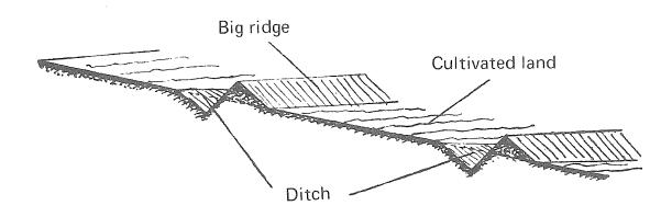
Ditches control erosion very well, but they must be cleaned out from time to time.
