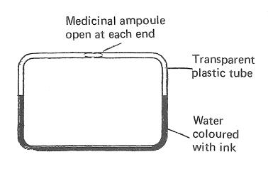
as shown in the drawing, putting the ampoule at the bottom. Protect the tube by strips of wood, except in the places shown in the drawing.
