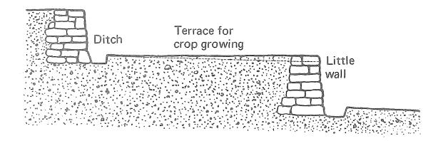
A ditch is made at the foot of the wall.
