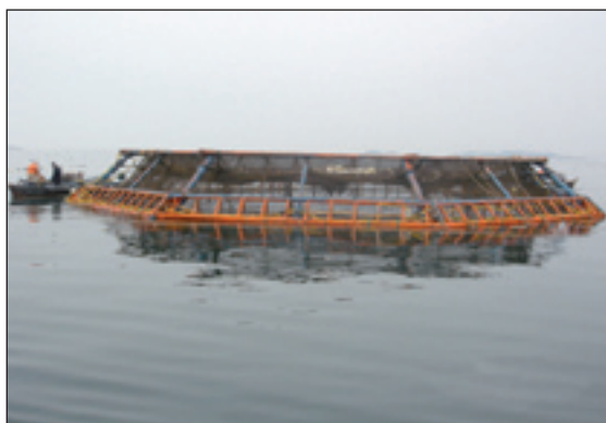
FIGURE 8 PDW submersible cage, manufactured by Fishery Machinery and Instrument Research Institute (FMIRI), Shanghai, China
