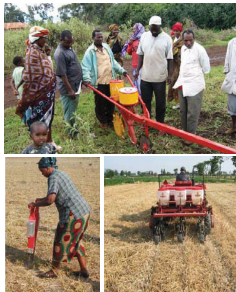
Figure 1. Direct seeding into mulch and moist soil by hand with jab planter, animal drawn seeder, and tractor mounted seeder
