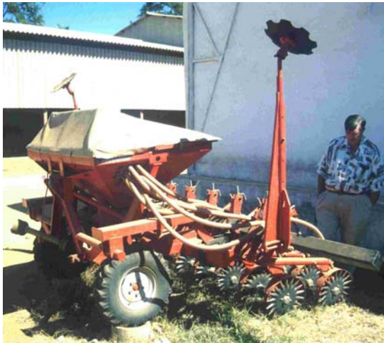
Plate 27 Rolling punch injection planter (starwheel planter). (T. Friedrich)
