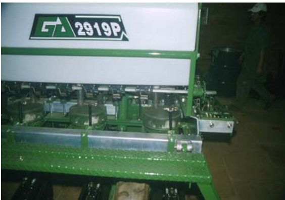
Plate 28 Detail of the inside of the seed container of a precision planter with seed plates to distribute the seeds. (V.H. de Freitas)
