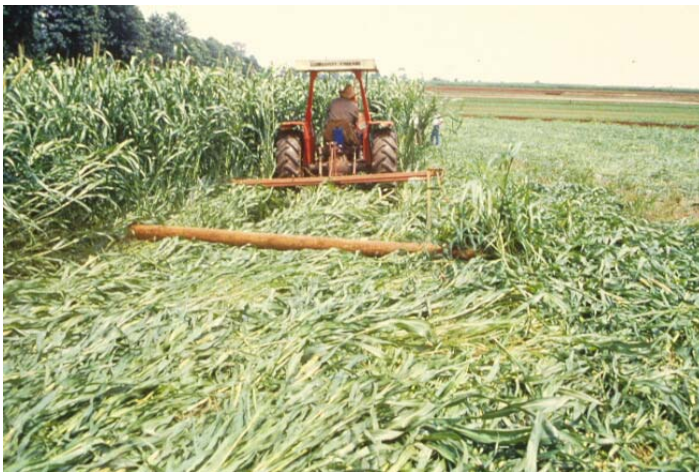
Plate 10 Metal tubes behind a tractor used as cover crop crusher.
