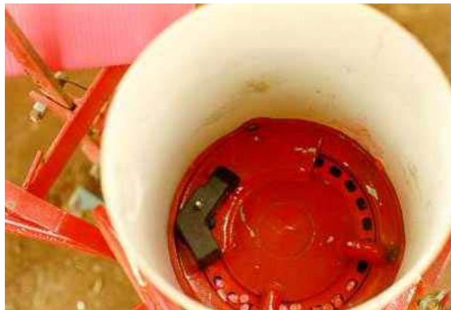
Plate 28 Detail of the inside of the seed container of a precision planter with seed plates to distribute the seeds. (V.H. de Freitas)
