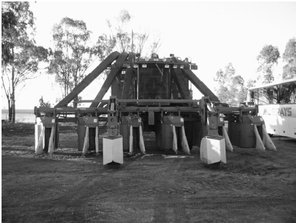
Picture 4: Six-row cotton picker adapted for controlled traffic farming at 3 m track width; additional support wheels in the front have been constructed by the farmer to support the header weight without double tyres (Jamie Grant/Australia) (photo by Friedrich).
