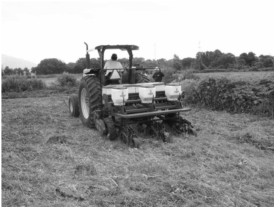
Picture 2: Direct seeding with minimal soil movement into heavy mulch cover (photo by Friedrich)
