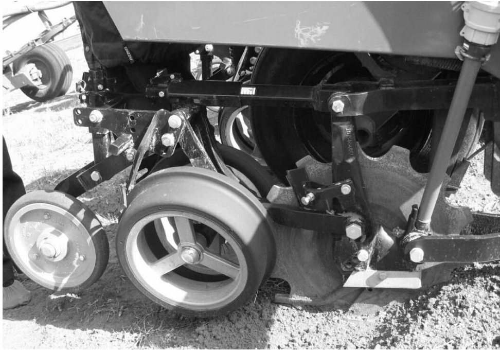
Picture 3: Cross slot®-furrow opener allowing direct seeding under no-till conditions into heavy mulch with minimum soil movement (photo by Friedrich)
