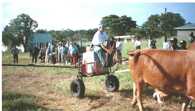
Fig.1 Demonstration of a Brazilian-made ride-on animal drawn sprayer in Uganda
