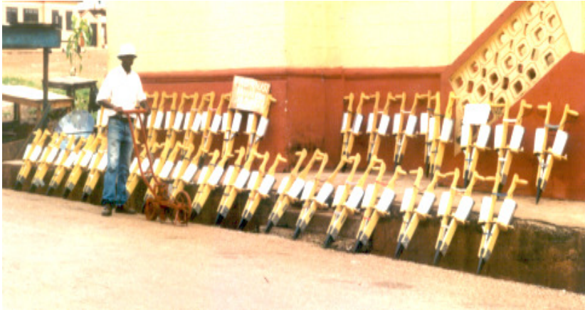
Fig.3 Hand jab-planters fabricated in Ghana
