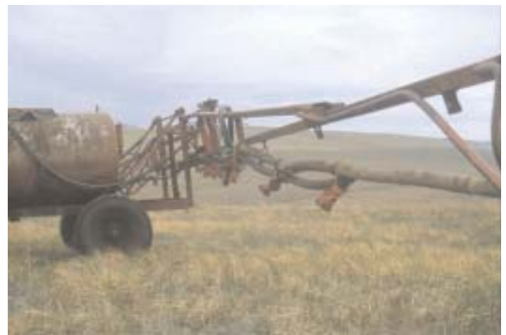
Photo 3. Badly maintained sprayer
