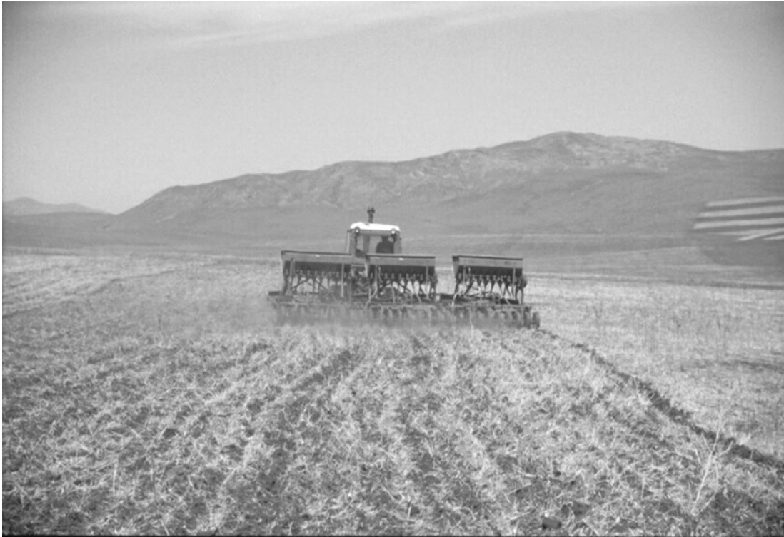
Fig. 2: Direct seeding with chisel furrow openers
