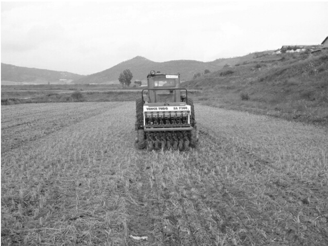
Fig. 3: Direct seeding with double disk furrow openers
