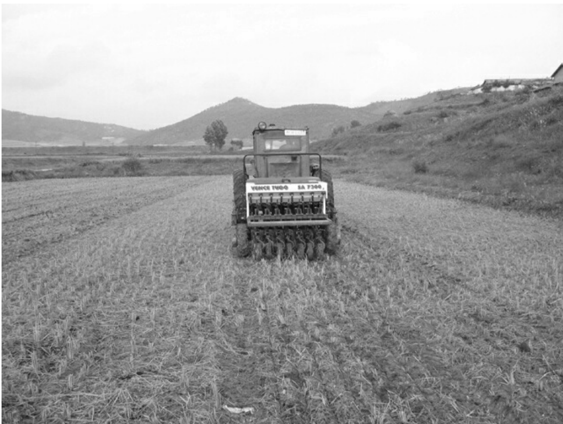
Fig. 3: Direct seeding with double disk furrow openers
