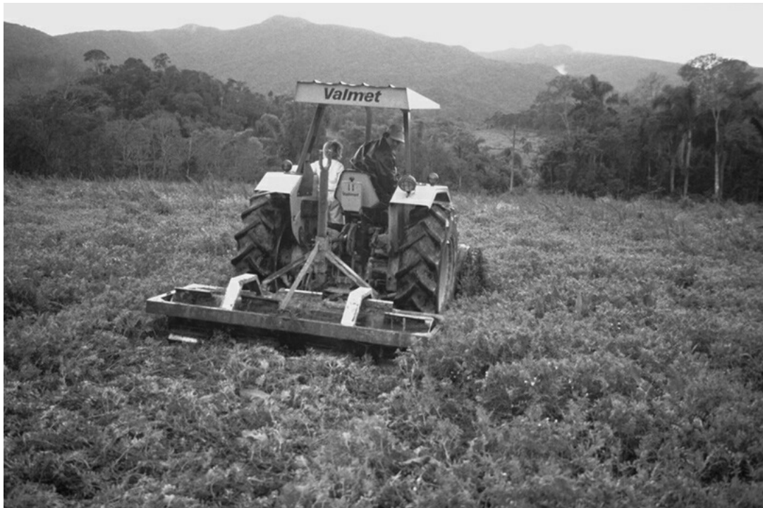
Fig. 4: Cover crop management with a knife roller
