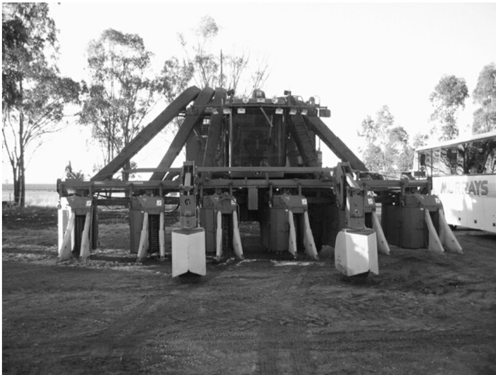
Fig. 6: Six row cotton picker prepared for controlled traffic farming on a 3 m track
