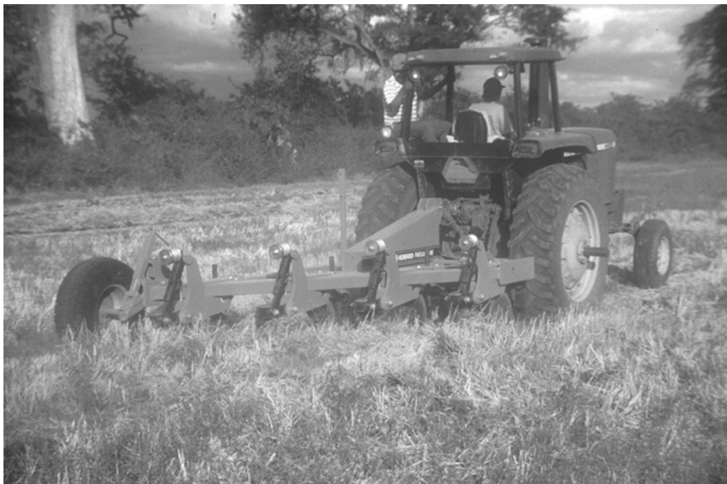
Fig. 1: Ripping with minimum soil disturbance with a Paraplow
